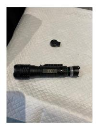
${\bf 5}$  -Screw the battery and battery holder back in the light
