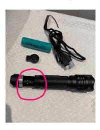
3- Place the battery in the battery holder. Make sure the negative end (-) is inserted into the light shaft, with the positive end (+) attached to the battery holder as shown.
